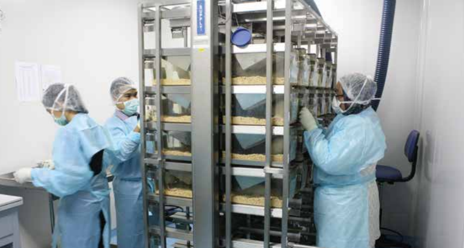
Another view of the experimental room equipped with individually ventilated caging (IVC) system
